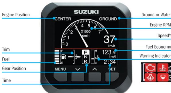
\* Speed sensor or GPS module will be required in order to display the speed.
